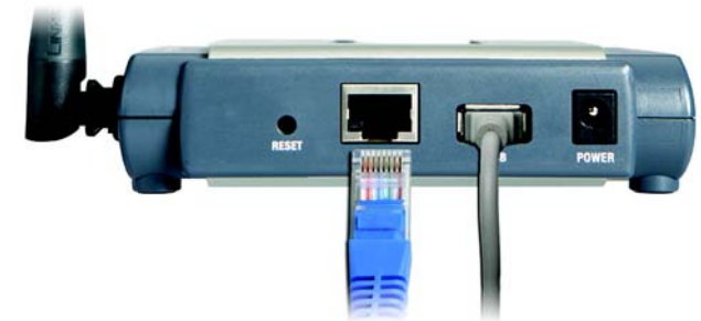
Figure 3-2: Connect to the Ethernet Port
