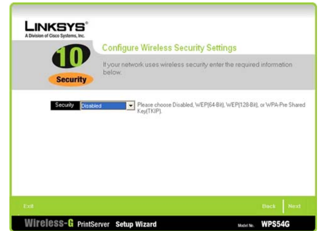
Figure 4-15: Wireless Security Settings - Disabled
