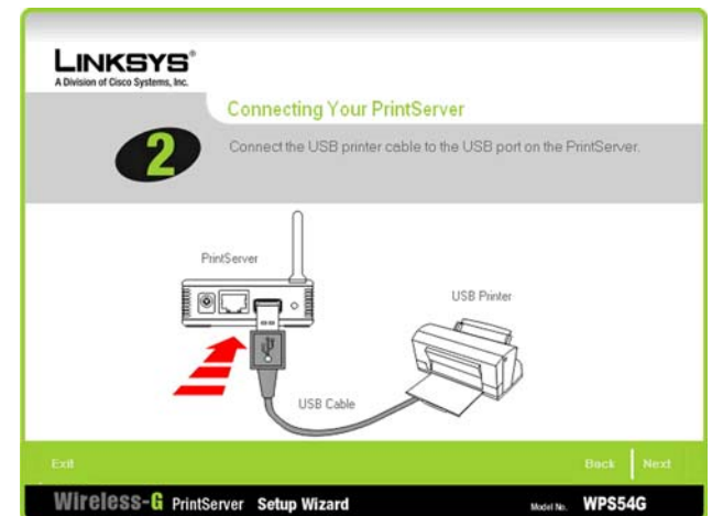
Figure 4-4: Connect the PrintServer to the Printer
