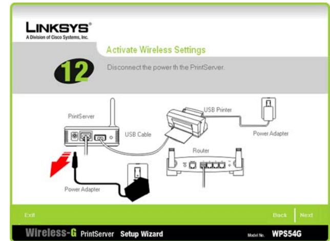
Figure 4-19: Disconnect power to the PrintServer
